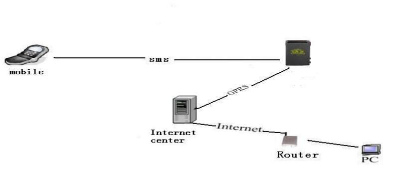
The tracker transfers GPS information to the network operator's machine room via GPRS first of all. Through wireless network, the GPS information is sent to internet and then a public IP associated with the router. The personal PC is connected with the internal network allocated by the router. In order to realize transferring GPS information to a personal PC correctly, the router must be able to transfer information received from WAN to the PCs in a LAN.
