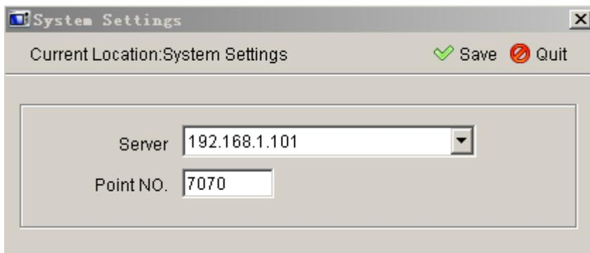
Attention: The corresponding system IP will be changed when you use the wired router, wireless router and wireless network card. IP will be shown in server field automatically, you only need to select one valid IP. If you the monitor software in the running status, pls stop running to change the IP address, it will be valid after changing and saving the system IP address.
